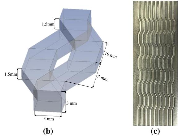
**Fig. 1.** (a) dimension, (b) Individual unit component, and (c) picture of corrugated channel.
