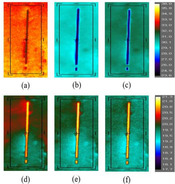
Figure 2. Temperature change of heated crack without moisture (a) Initial heating, (b) After 5 minutes of heating, (c) After 10 minutes of heating, (d) After 15 minutes of cooling, (e) After 30 minutes of cooling, and (f) After 60 minutes of cooling.
