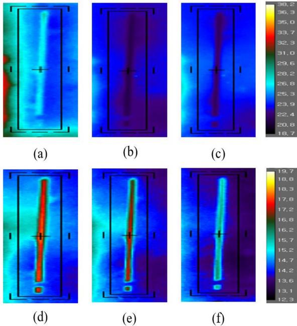
Figure 3. Temperature change of heated crack with moisture (a) Initial heating, (b) After 5 minutes of heating, (c) After 10 minutes of heating, (d) After 15 minutes of cooling, (e) After 30 minutes of cooling, and (f) After 60 minutes of cooling
