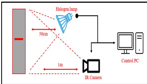
Figure 1. Experimental setup to detect the temperature differences between defect and non-defect regions.
