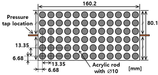
Figure 2. Cross section of test section
