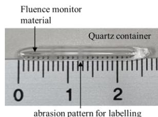
Fig. 3. Fabricated FM element using quartz container.
