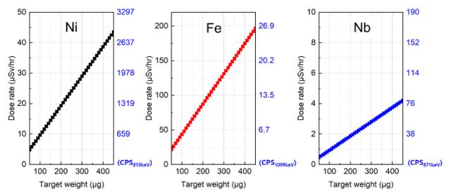
Fig. 2. Dose rate and expected cps based on FM weight. NAAPro [3] was used in the calculation. Irradiation and cooling period was set to be 56 days and 1 year respectively.
