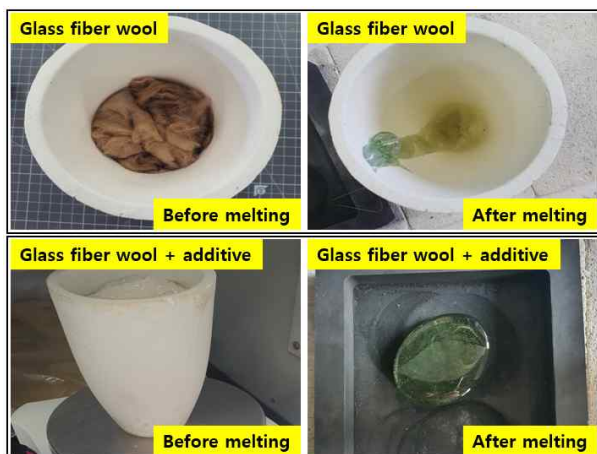
Fig. 4. Picture of melted glass fiber wool: (upper) only glass fiber wool (bottom) glass fiber wool with additive.
