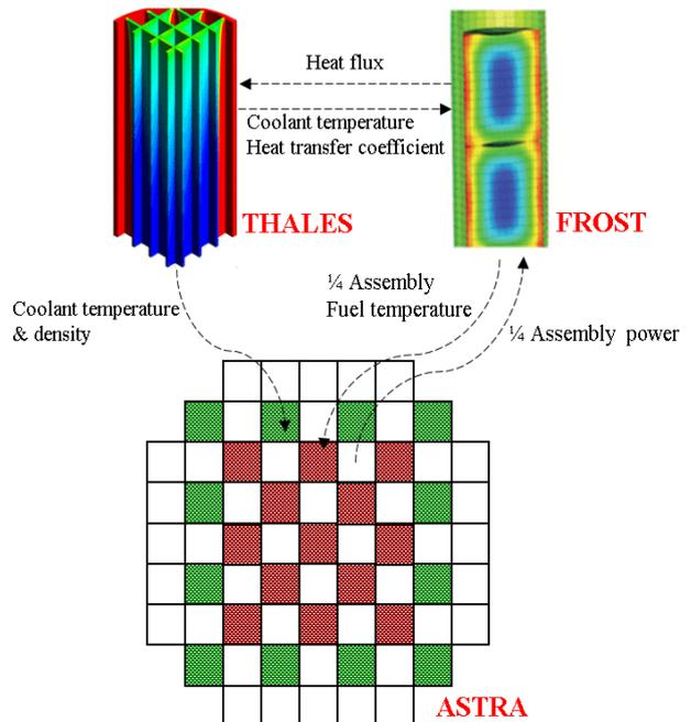
Fig. 1. Main flow chart of the CHASER code system
