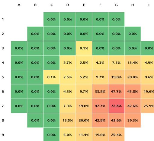
Fig. 5. Percentage of DNBR decrease compared to initial DNBR for Each Fuel Assembly (CHASER-SPACE)
