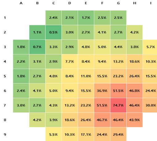
Fig. 4. Percentage of DNBR decrease compared to initial DNBR for Each Fuel Assembly (CHASER)
