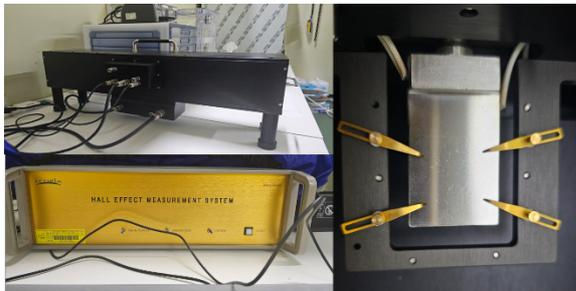
Fig. 3. Hall Effect Measurement system at KAERI
