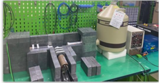
Fig. 4. Positron Annihilation Spectroscopy system at KAERI.
