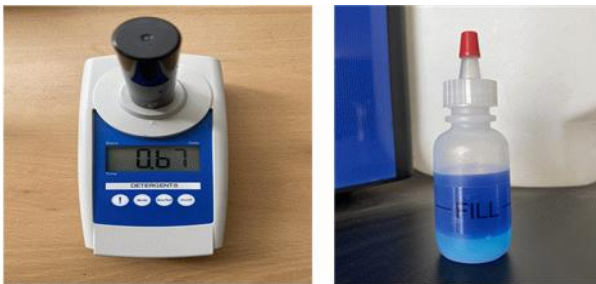
Fig. 1. Anionic surfactant measurement scene and sample bottle injected with measurement solution
