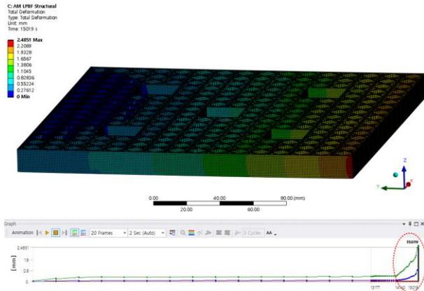
Fig. 2. Total deformation for base removal.
