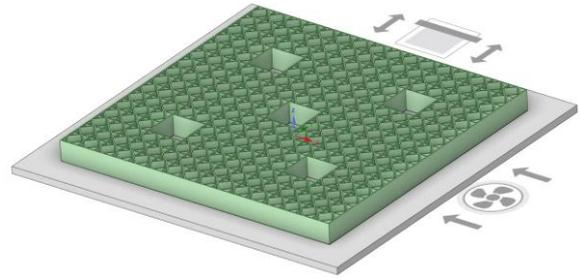
Fig. 1. Setup of spacer grid model for AM simulation
