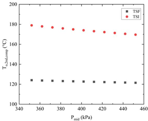
Fig. 6. Temperature of the refrigerant at the exit of the second compressor at TSF and TSI.
