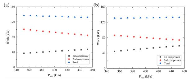
Fig. 5. Power consumption of the compressors at TSF and TSI.
