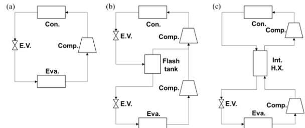
Fig. 1. Three different heat pump cycles. (a) Single-stage compression cycle(SC), (b) two-stage compression cycle with a flash tank(TSF), (c) two-stage compression cycle with an internal heat exchanger(TSI).
