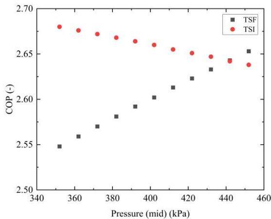
Fig. 4. The trend of COP variation according to the increase of intermediate pressure at TSF and TSI.
