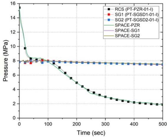
Fig. 3. SPACE prediction of system pressure
