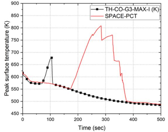
Fig. 5. SPACE prediction of peak surface temperature
