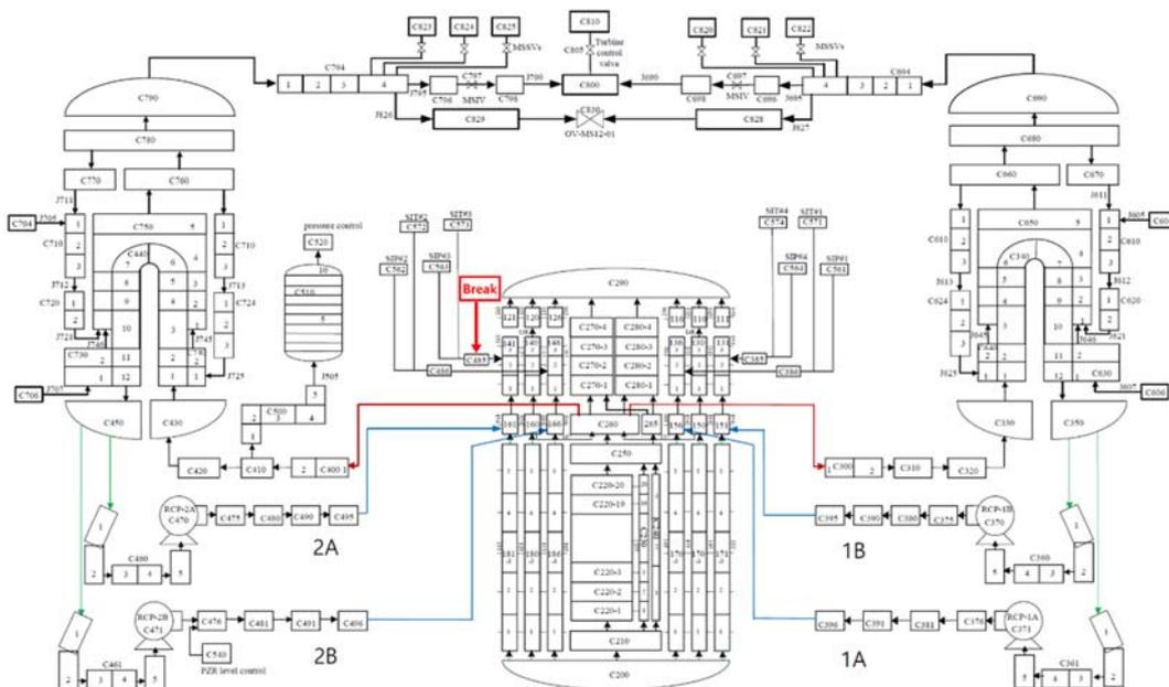
Fig. 1. Nodalization of the SPACE input model for ATLAS test facility
