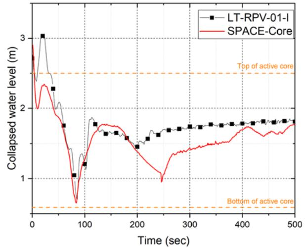
Fig. 8. Core collapsed level (Case 2,  $M=1.0$ ,  $C=1.0$ )
