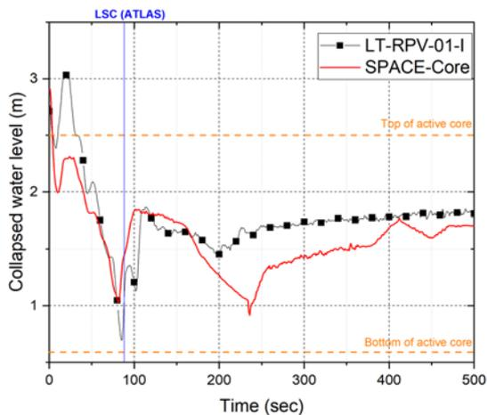
Fig. 4. SPACE prediction of core collapsed level
