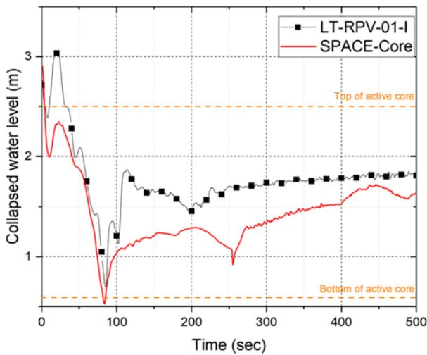
Fig. 6. Core collapsed level (Case 1,  $M=1.22$ ,  $C=0.88$ )
