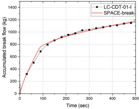
Fig.2. SPACE prediction of the accumulated break flow
