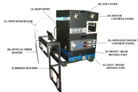
Fig2. Picture of OFPS's main part and components
