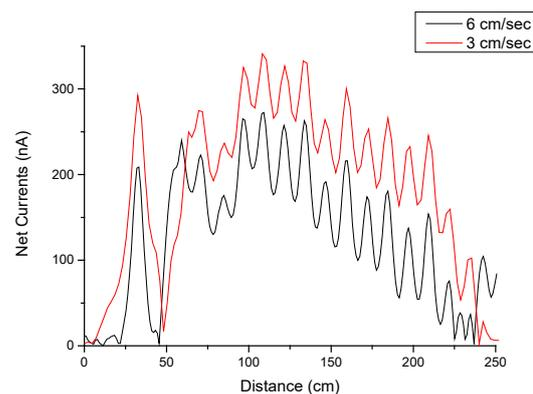
Fig4. Effect on the velocity of the detector moving (black) 6cm/sec (red) 3mm/sec
