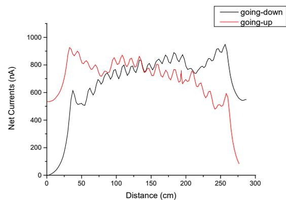
Fig3. Effect on the direction of the detector moving (black) going-down (red) going-up
