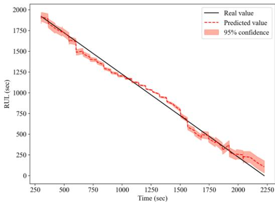
Fig. 5. IGBT RUL prediction results for test data in the model of group 3 (in the case of 15 sequences).
