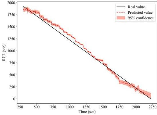
Fig. 3. IGBT RUL prediction results for test data in the model of group 1 (in the case of 15 sequences).
