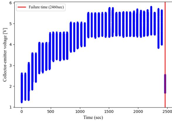
Fig. 2. Collector-emitter voltage values and failure time over time.
