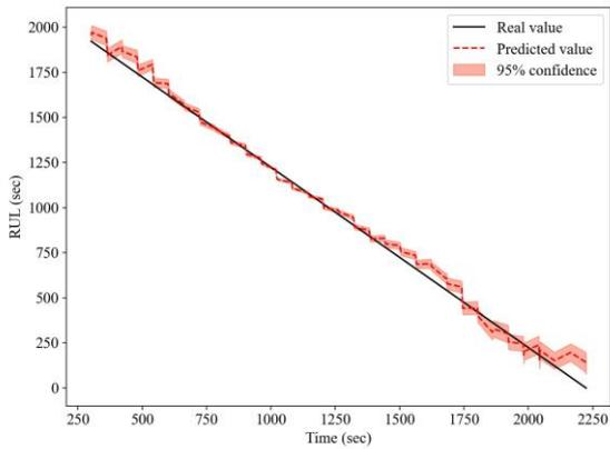
Fig. 4. IGBT RUL prediction results for test data in the model of group 2 (in the case of 15 sequences).
