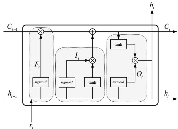
Fig. 1. Structure of LSTM cell [1].
