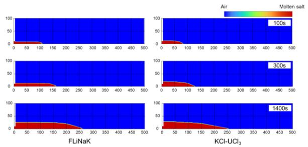
**Fig. 5.** The spreading behavior of FLiNaK and KCl-UCI<sub>3</sub> on flat SS304 at 100s, 300s, and 1400s.
