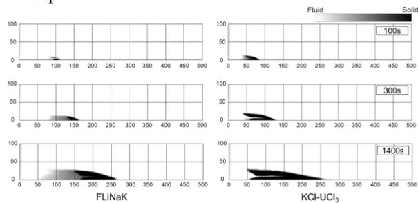
**Fig. 6.** The Solidification of FLiNaK and KCl-UCI<sub>3</sub> on flat SS304 at 100s, 300s, 1400s.
