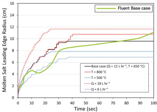
**Fig. 3.** The spreading of FLiNaK on flat SS304 compare with MELTSPREAD and Fluent.
