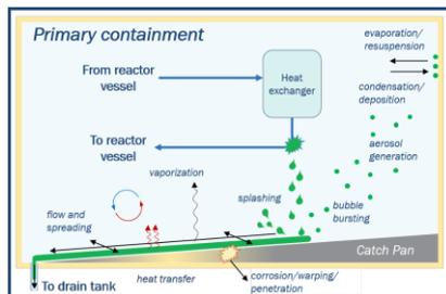
**Fig. 1.** A schematic of molten salt leaking from the MSR and spilling onto the catcher.
