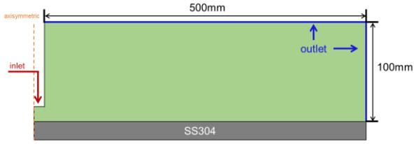
**Fig. 2.** Domain of leaking molten salt numerical simulation.
