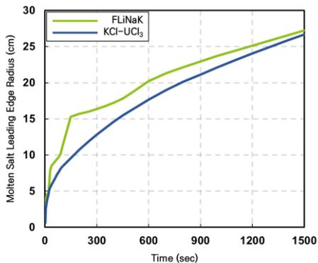
**Fig. 4.** The spreading of FLiNaK and KCl-UCI<sub>3</sub> on flat SS304 with Fluent.
