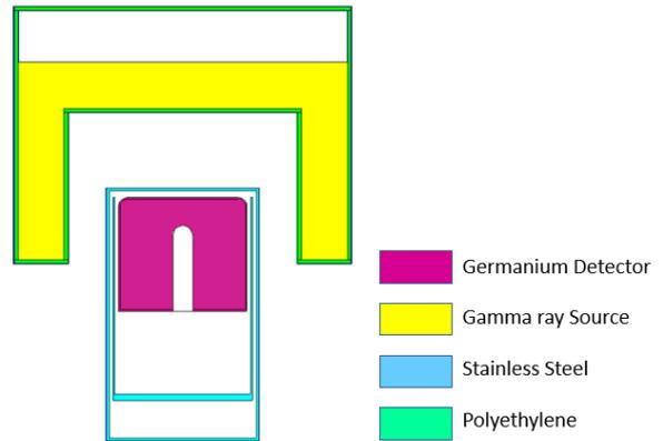
Fig. 1. MCNP Geometry Model
