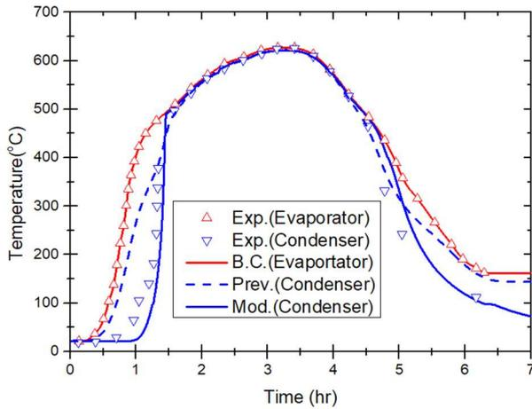
Fig. 2. Simulated wall temperature results with the evaporator wall temperature boundary condition.
