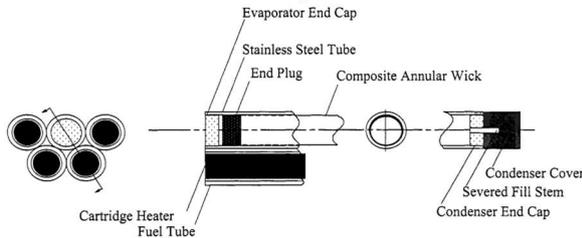
Fig. 1. SAFE-30 Experimental apparatus[3]
