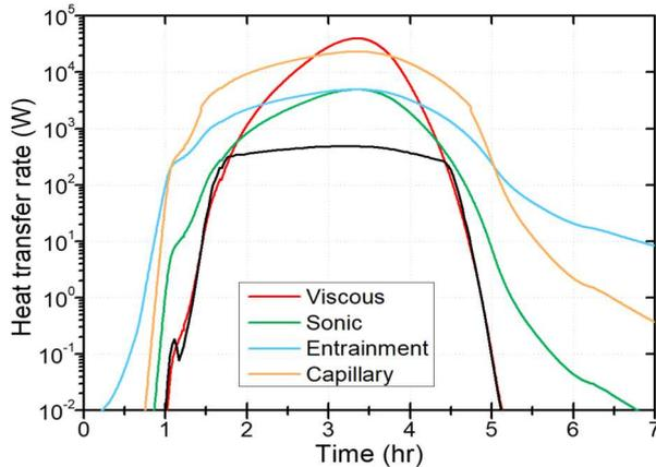
Fig. 4. Simulated vapor heat transfer rate and limit results with B.C.1
