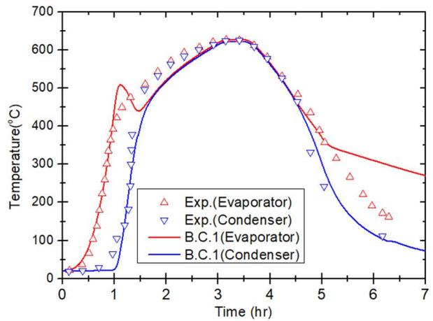
Fig. 3. Simulated wall temperature results with B.C.1
