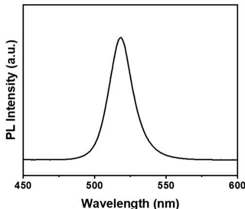
Fig. 1. PL spectrum of CsPbBr<sub>3</sub> nanocrystals.
