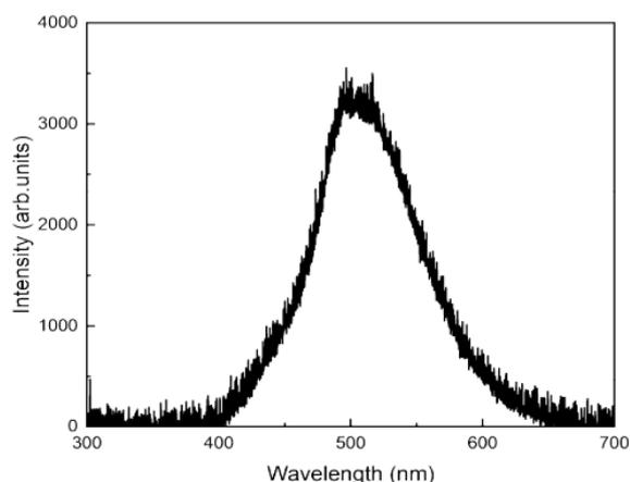
Fig. 4. Radioluminescence spectrum of flexible scintillator composed of PMMA and CsPbBr<sub>3</sub> nanocrystals...
