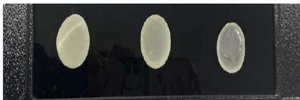
Fig. 2. Photograph of flexible scintillator composed of PMMA and CsPbBr<sub>3</sub> nanocrystals.
