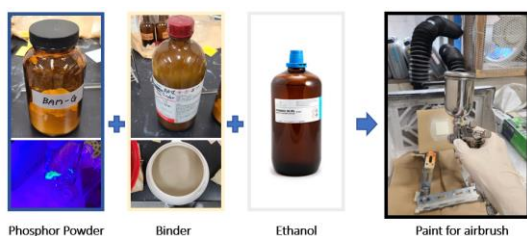
Fig. 2. BAM:G Phosphor paint mixing and spraying process
