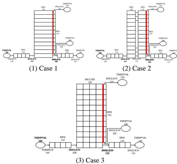
Fig. 2. MARS-LMR nodalization of SUPERCAVNA experiment.
