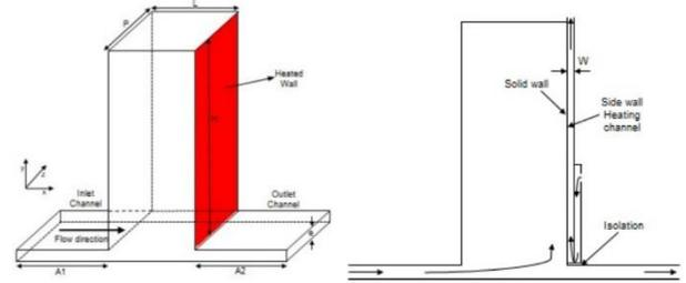
Fig. 1. Geometry and flow direction of SUPERCANVA facility.
