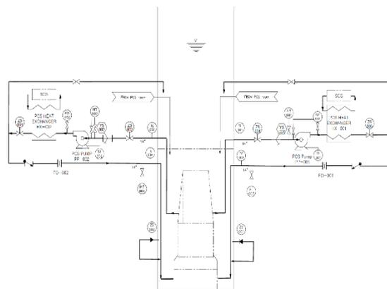
Figure 2. Flow Diagram of the Optimized PCS
