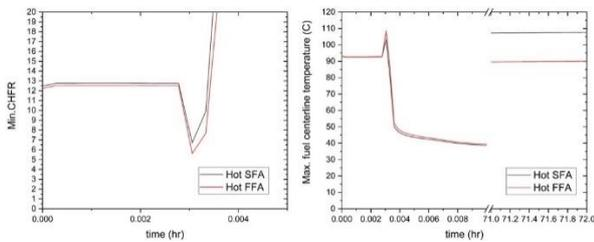
Figure 6. Minimum CHFR and Maximum Fuel Centerline Temperature vs Time
