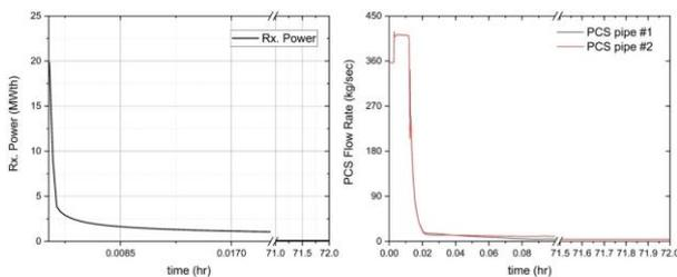
Figure 4. Reactor Power and PCS Flowrate vs Time
