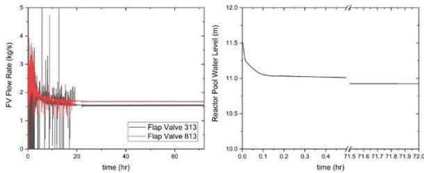
Figure 5. Flap Valve flowrate and Pool Level vs Time
