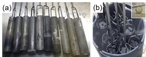
Fig. 2. Photos of SS wire mesh baskets used for the immersion of the fuel: (a) side view and (b) top view (inset image: cross-section of metallic simfuel).
