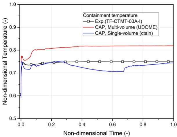
Fig. 5. Containment temperature in the C1.2 test
