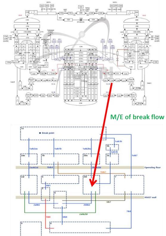
Fig. 2. Nodalization for the SPACE-CAP code calculation
