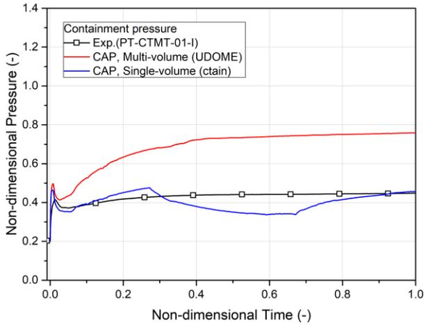
Fig. 4. Containment pressure in the C1.2 test
