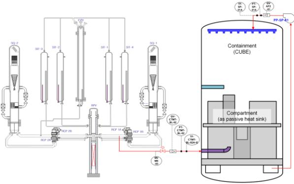
Fig. 1. A schematic diagram for the ATLAS-CUBE test
