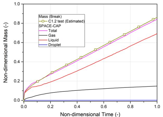
Fig. 3. Integrated mass of the break flow in C1.2 test
