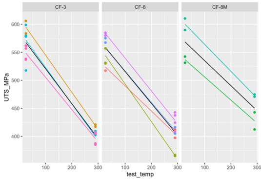
Fig. 1. UTS variation with measurement temperature for unaged specimens.
