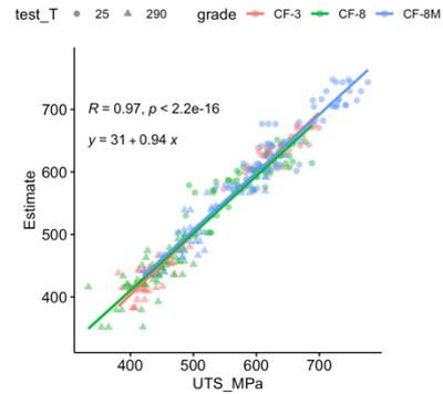
Fig. 3. Predictive performance of the developed multilevel model on the properties of aged specimens.
