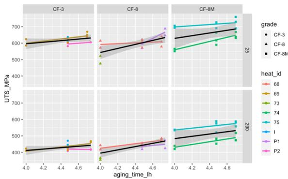
Fig. 2. UTS variation of specimens aged at 320°C for various times. Aging times have been converted to  $\log_{10}$ .
