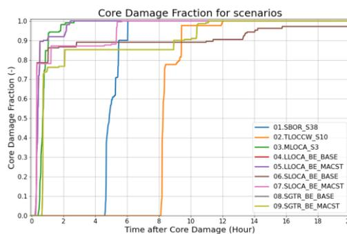
Fig. 4. Fraction of damaged core nodes from MAAP5 calculation.
