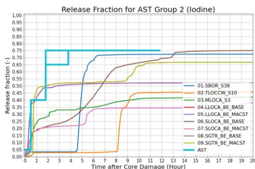
Fig. 2. Release fraction of AST Group 2 (Iodine) to in-containment relative to initial in-core inventory.
