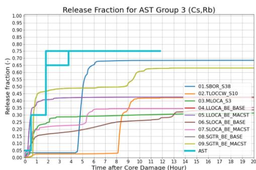
Fig. 3. Release fraction of AST Group 3 (Cs, Rb) to in-containment relative to initial in-core inventory.
