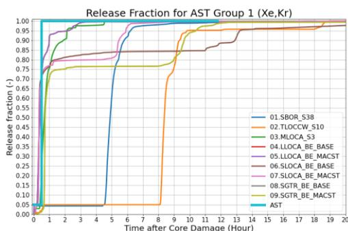
Fig. 1. Release fraction of AST Group 1 (Xe, Kr) to in-containment relative to initial in-core inventory.
