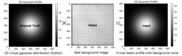
Fig. 1. Process of generating a dataset of virtual beam profile with background noise
