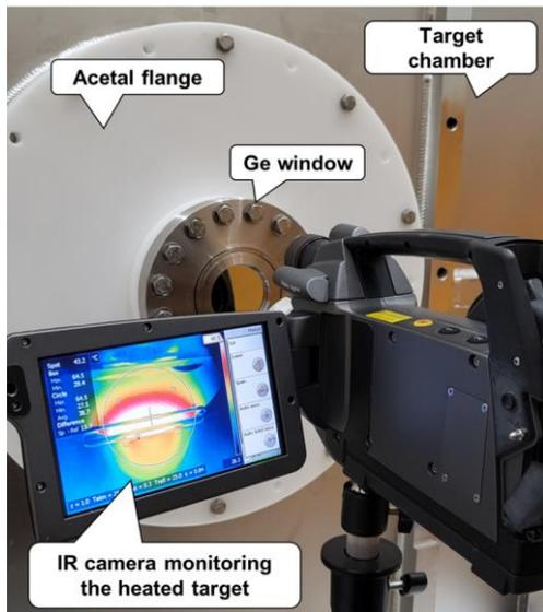
Fig. 3. Experiment setup including Ge window, IR camera, and the target chamber during the experiment
