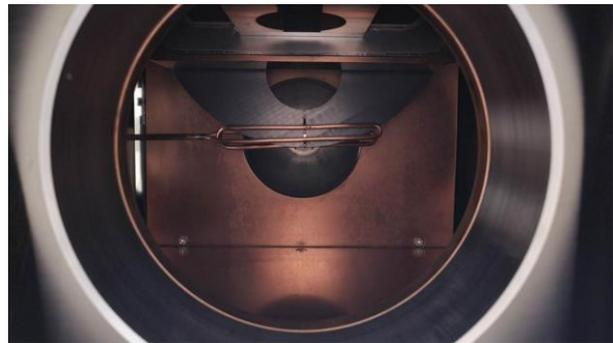
Fig. 2. Inner view of the target chamber showing the copper coil and the graphite target
