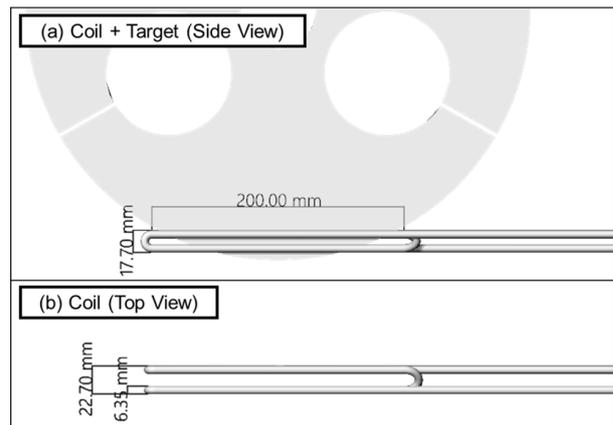
Fig. 1. Copper coil design for the experiment
