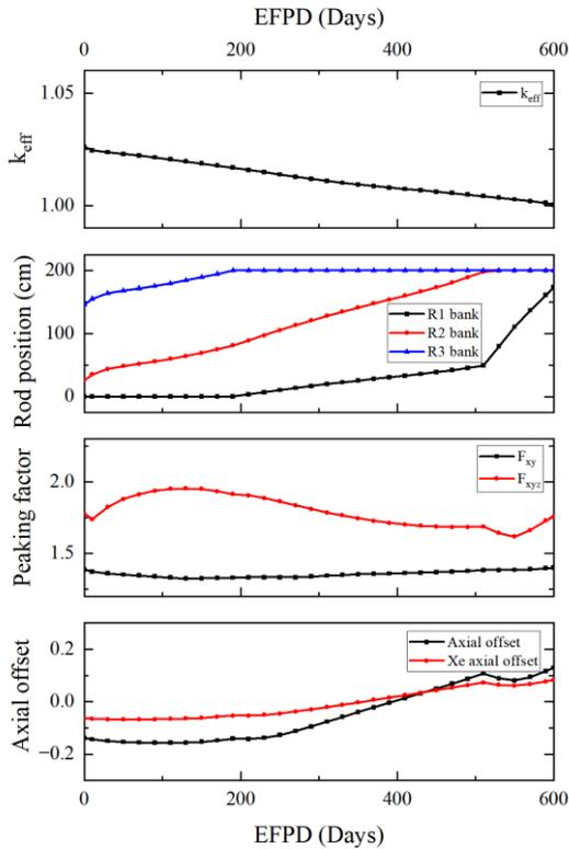
**Figure 6. Changes of core parameters of the core at the equilibrium cycle**
