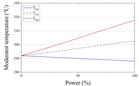
Figure 5. Change of moderator temperature with respect to the power output
