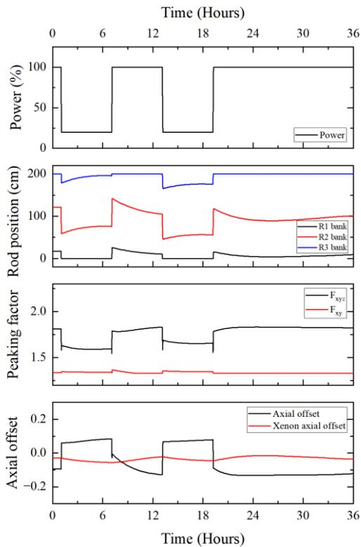
**Figure 8. Changes of core parameters during unusual load-following at the equilibrium cycle MOC**
