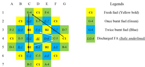
Figure 3. The 3-batch configuration of the core
