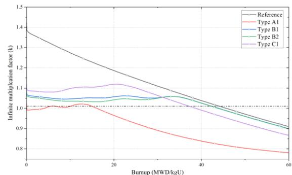
Figure 2. The infinite multiplication factors ( $k_{inf}$ ) of the optimized fuel assemblies with respect to burnup
