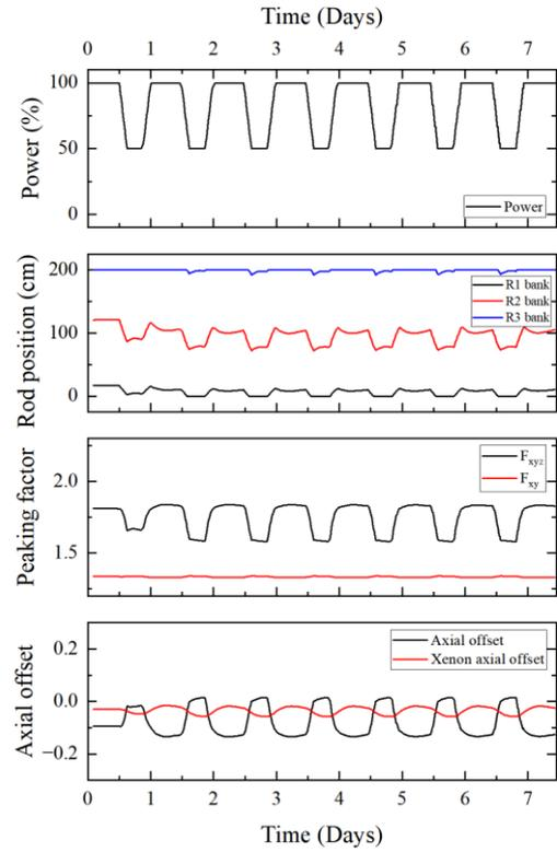
**Figure 7. Changes of core parameters during usual load-following at the equilibrium cycle MOC**
