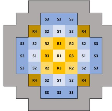
Figure 4. Configuration of the control rod banks
