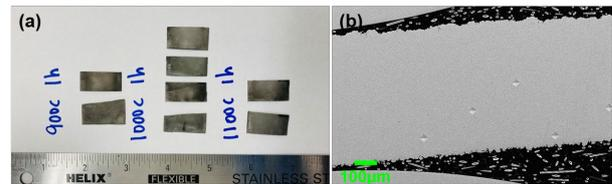
Fig. 4. (a) Photograph and (b) cross-sectional SEM image of free-standing NFA flats produced using ball-milled 14YWT powders.
