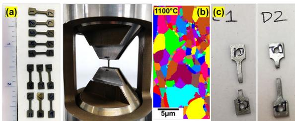
Fig. 3. (a) Photographs of SSJ3 type tensile specimens and tensile testing facility, (b) EBSD data showing grain size distribution for NFA specimen annealed at 1100 °C, and (c) photographs of tensile samples after testing.
