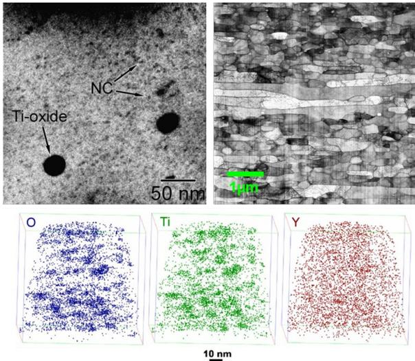
Fig. 1. TEM images showing microstructure of 14YWT and atomic probe tomography image of nanocluster in 14YWT [2].
