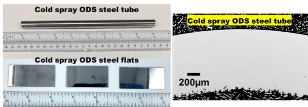
Fig. 2. (Left) Photographs of an NFA tube and flat samples produced by CST and (Right) cross-sectional SEM image of the tube sample, exhibiting high-density microstructure.
