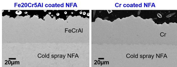
Fig. 5. (Left) FeCrAl coated NFA flat and (Right) Cr coated NFA flat samples produced using CST.
