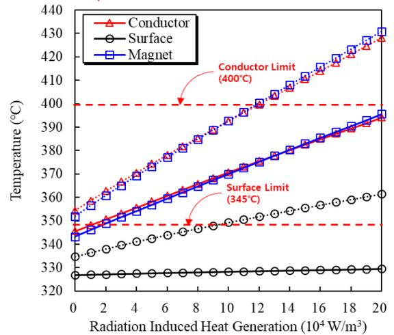
Fig. 5. Maximum temperature vs irradiation heat:
