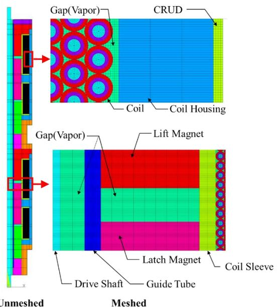
Fig. 2. Analysis model of the IV-CEDM
