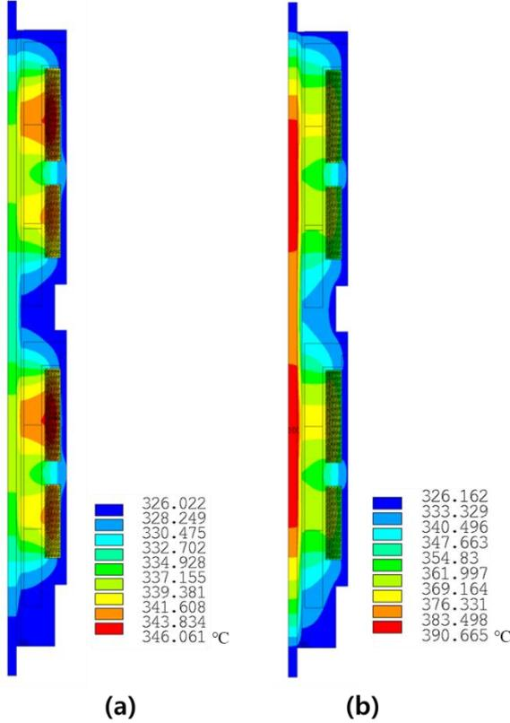
Fig. 3. Temperature distribution of the IV-CEDM ( $t_{crud}=0.1$  mm,  $I_{coil}=6$  A,  $v_{coolant}=0.2$  m/s):
