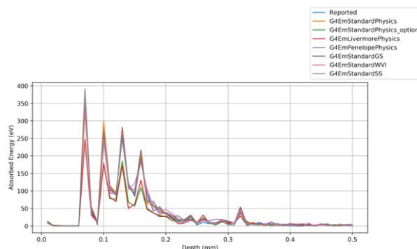
Fig 3. The absorbance data of Co film-MgO substrate material, for seven physics models. The x axis stands for every 0.1mm in the substrate.
