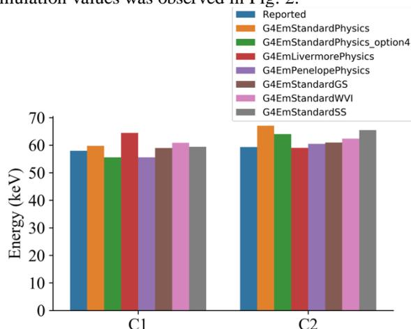
Fig. 2. The X-ray output spectra from characteristic radiation, compared with the empirical data (reported) and the simulation data (other models starts with 'G4'). C1: lower characteristic radiation energy, C2: higher characteristic radiation energy.
