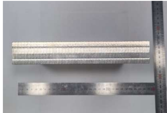
Fig. 1. Side view of Ni-cladded Type 316H stainless steel after milling.
