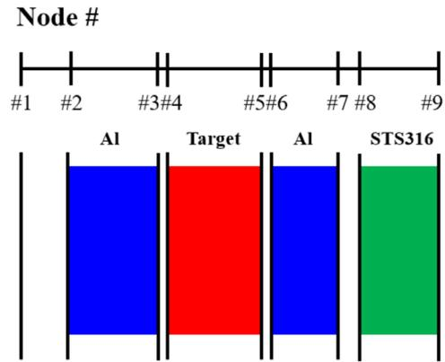
Fig. 1. One-dimensional order of materials arranged from the center of the irradiation hole and the divided node numbers.
