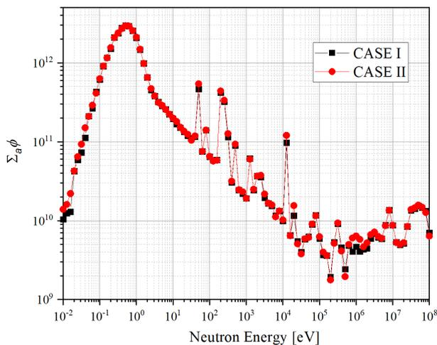
Fig. 3. Neutron absorption reaction rates along with the neutron energy.
