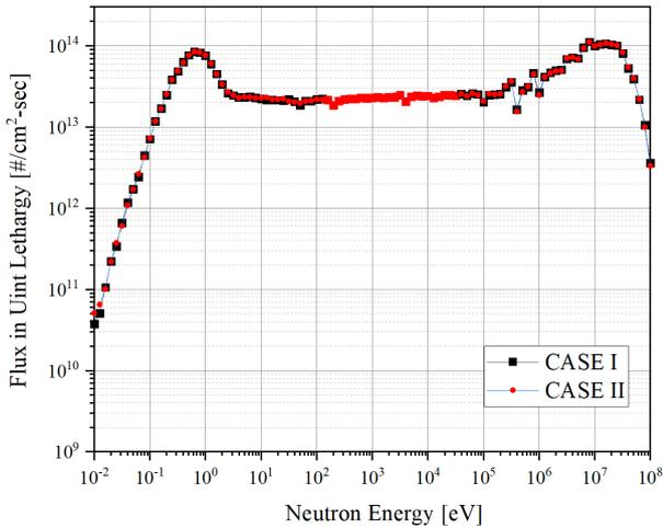
Fig.2. Neutron Flux distributions in unit lethargy along with the neutron energy.
