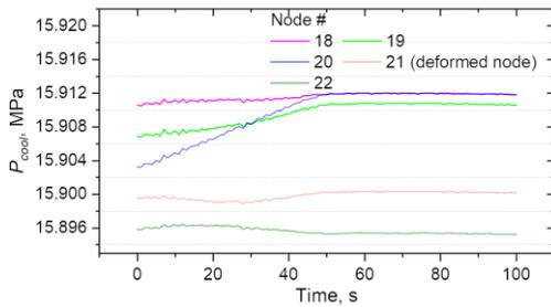
Fig. 4. Change of hot channel coolant pressure ( $P_{cool}$ ) at around deforming fuel node (#21)
