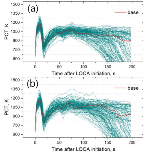
Fig. 5. Evolution of 124 PCT curves during LOCA, evaluated with (a) no blockage models and (b) blockage models
