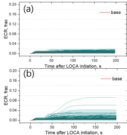
Fig. 6. Evolution of 124 CP-ECR curves during LOCA, evaluated with (a) no blockage models and (b) blockage models
