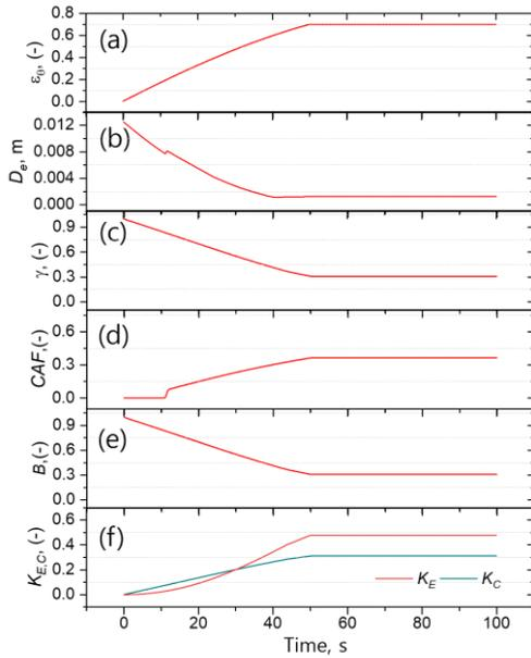
Fig. 2. Evolution of (a) cladding hoop strain ( $\epsilon\theta$ ), (b) equivalent hydraulic diameter ( $D_e$ ), (c) porosity ( $\gamma$ ), (d) contact area fraction ( $CAF$ ), (e) flow area ratio ( $B$ ), (f) form loss coefficient of expansion ( $K_E$ ) and contraction ( $K_C$ )
