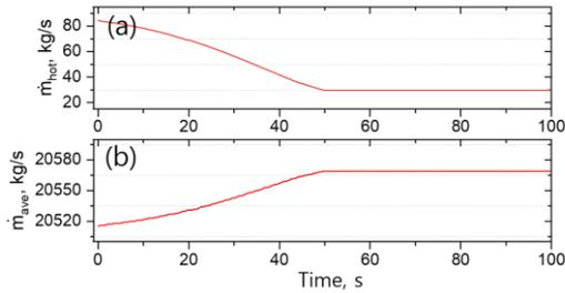
Fig. 3. Change of mass flow rate at (a) hot channel ( $\dot{m}_{hot}$ ) and (b) average channel ( $\dot{m}_{ave}$ )
