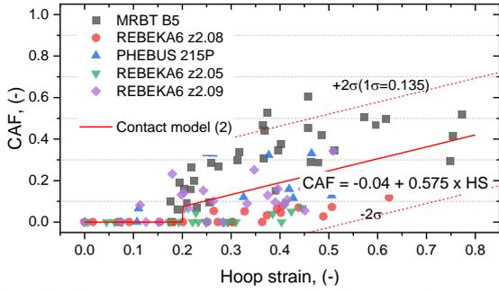
Fig. 1. Contact area fraction (CAF) as a function of cladding hoop strain ( $hs$ ) [9].
