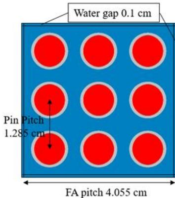
Fig. 3. The cross-sectional view of the  $\text{UO}_2$  fuel assembly
