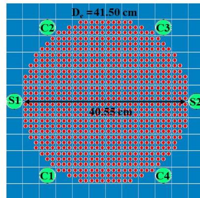
Fig. 4. The  $\text{UO}_2$  fuel-loaded core configuration
