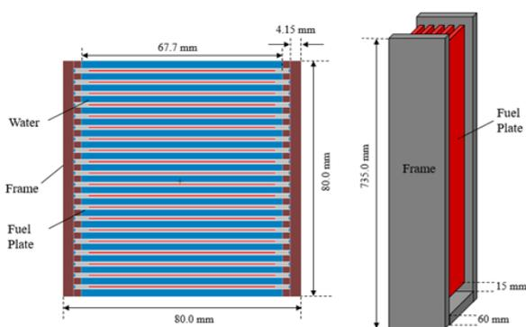
Fig. 8. The configuration of the U-7Mo fuel assembly
