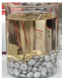
Fig. 1. Purification of \text{AlCl}_3 -urea DES (molar ratio: 1.4:1) after synthesis
