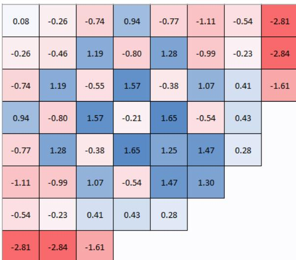
Fig 3. Radial power distribution before adjustment are displayed. The maximum and RMS power error is -2.81%, and 1.21% respectively.
