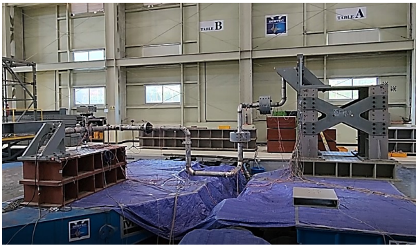
Fig. 1. Experimental set up for shaking table test consisting stainless steel specimen.
