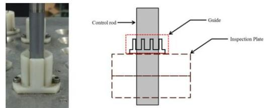
Fig. 4. Inspection plate guide.
