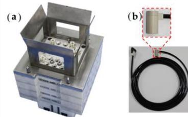
Fig. 3. Inspection plate (a) and sensor probe (b).
