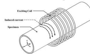
Fig. 5. Induced current on a tube specimen without cracks.
