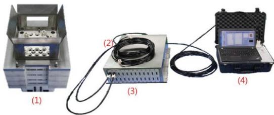
Fig. 2. RCCA inspection system: (1) inspection plate, (2) exciting coil, (3) multiplexing unit, (4) interface with computer and software.
