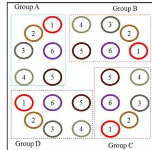
Fig. 9. Grouping of control rods for multiplexing process.
