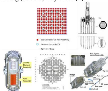
Fig. 1. Fuel rod assembly and rod cluster control assembly.
