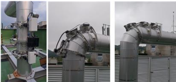
Fig. 9. A prototype of robot mounted on the exterior wall of pipe.
