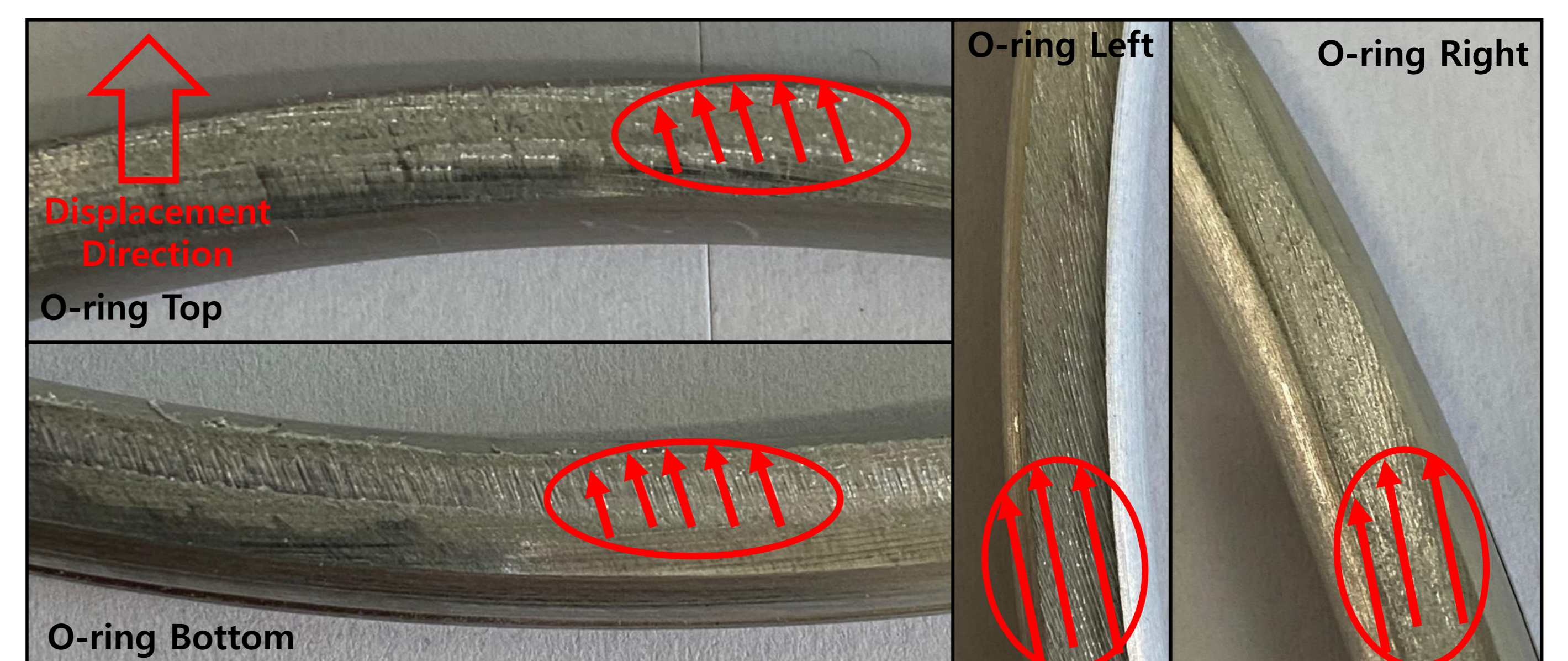
Fig. 5 O-ring after differential pressure test by applying displacement
