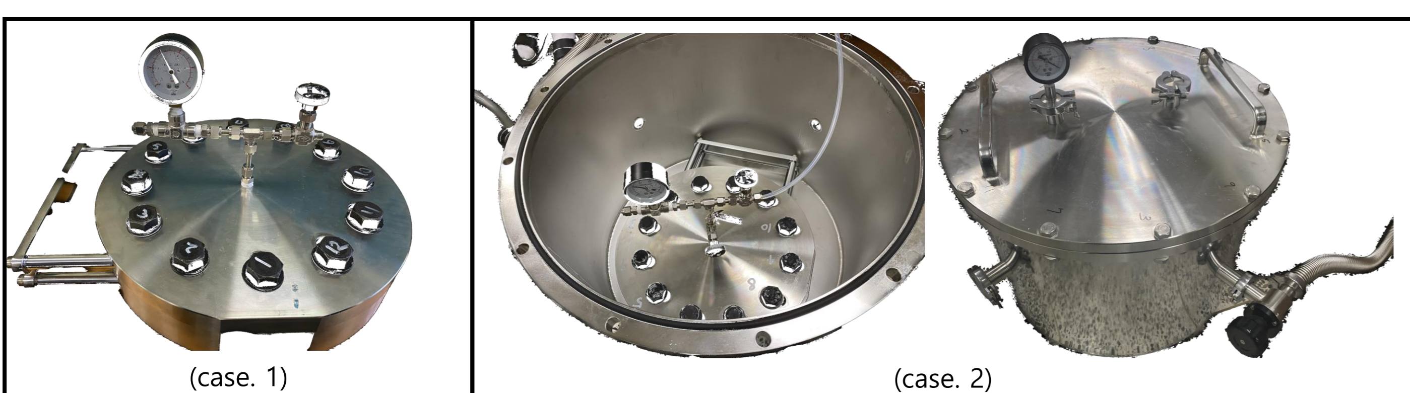
Fig. 3 (case. 1) Pressure drop test of atmospheric pressure, (case. 2) helium leak test of vacuum pressure
