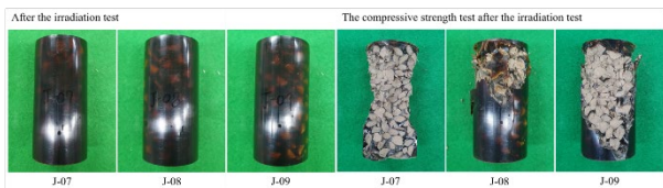
Fig. 4. Images of polymer waste form. (a) After irradiation test, (b) Compressive strength test after irradiation test.
