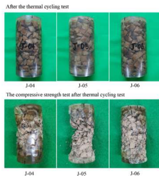
Fig. 4. Images of polymer waste form. Before compressive strength test, After compressive strength test.
