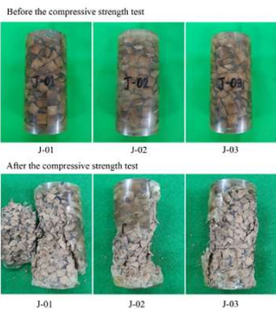
Fig. 3. Images of polymer waste form. Before compressive strength test, After compressive strength test.
