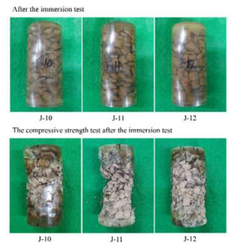
Fig. 6. Images of polymer waste form. Before compressive strength test, After compressive strength test.
