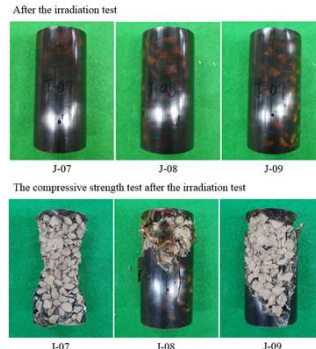
Fig. 5. Images of polymer waste form. Before compressive strength test, After compressive strength test.
