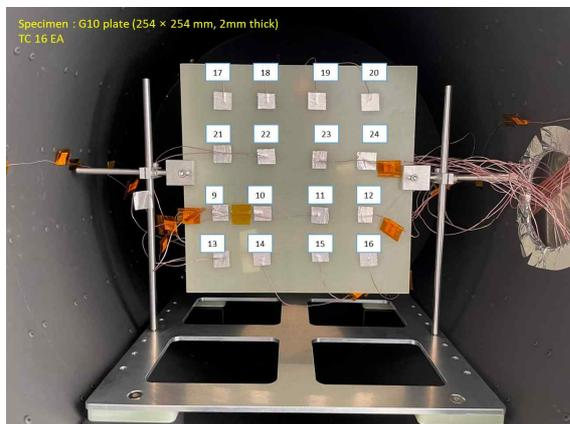
Fig. 5. The simulated specimen and attached 16 thermocouples
