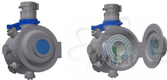
Fig. 1. Overall design of the thermal-vacuum chamber for space environment simulation
