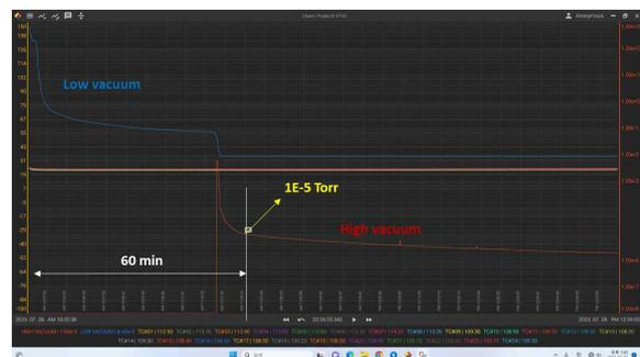
Fig. 3. The vacuum test of the space radiation environment simulator
