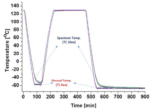
Fig. 6. The thermal cycling and temperature uniformity
