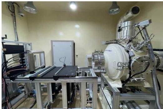
Fig. 2. The installation of the space radiation environment simulator at TR102 facility.
