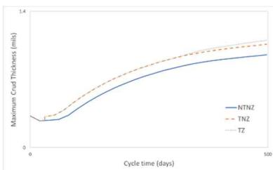
Fig. 3. Maximum crud thickness versus cycle time
