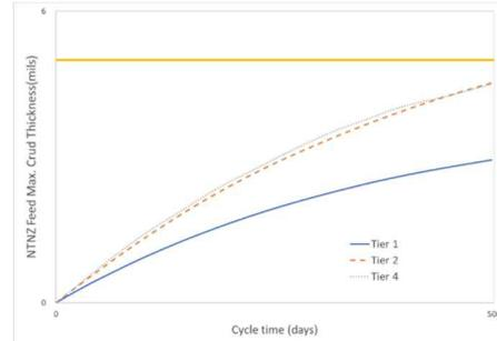
Fig. 9. Feed maximum crud thickness about Tier 1, 2 and 4 in NTNZ case
