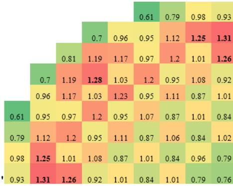
Figure 12: Radial Power Distribution (Nodal Model)
