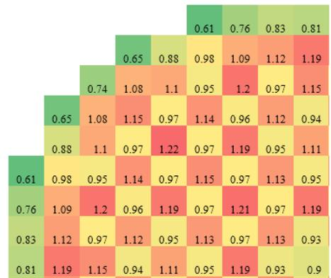
Figure 13: Radial Power Distribution (DCD)
