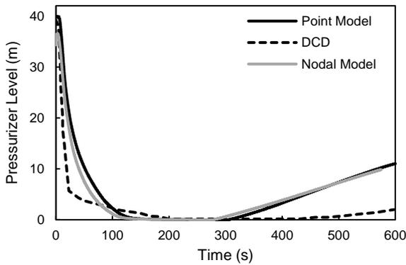
Figure 19: Pressurizer Level (Nodal Kinetics)
