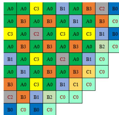
**Figure 3: Fuel Loading Pattern for a Quarter Core**
