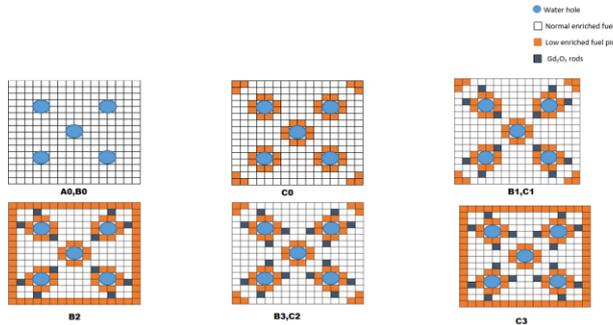
Figure 4: First Cycle FAs Configurations
