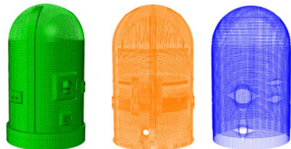
(a) containment (b) rebar (c) tendon
