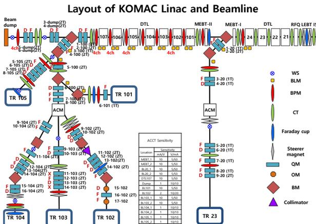
Fig. 1. layout of the 100 MeV linear accelerator at KOMAC.
