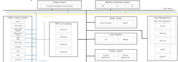
Fig. 3. The Block diagram of the KOMAC control system.
