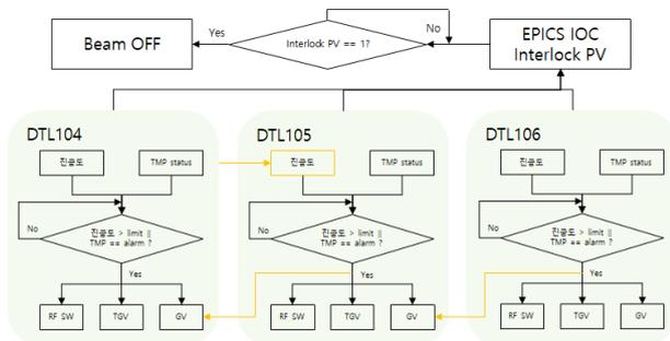
Fig. 5. The interlock sequence of the vacuum system.
