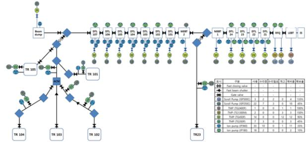
Fig. 2. The Block diagram of the vacuum system at KOMAC.
