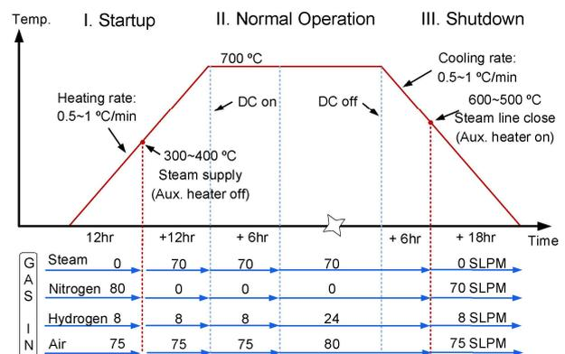
Fig. 2. Example of an operating procedure for a 6.0 kW capacity HTSE system [4].
