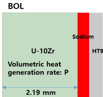
Fig. 1 Schematic cross-section of the metallic fuel
