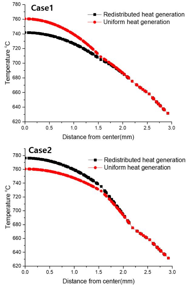
Fig. 5. Temperature distribution of Case 1 and Case2 with consideration of radial heat generation rate distribution.
