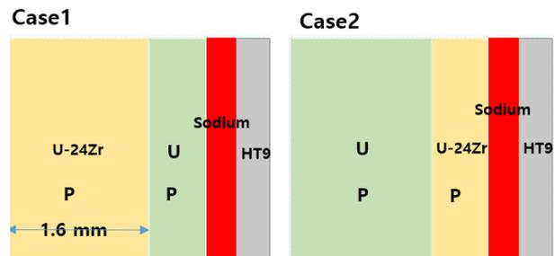
Fig. 2. Schematic cross-section of the metallic fuel: Case1 and Case 2
