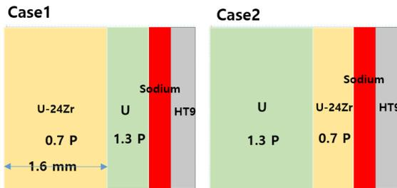
Fig. 4. Schematic cross-section of the metallic fuel: Case1 and Case2
