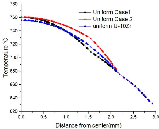
Fig. 3. Temperature profile of metallic fuel with uniform heat generation: Uniform Zr distribution, Case1, Case2.
