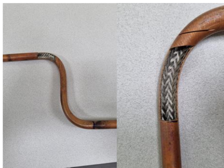
Fig. 2. Braided wire wick structure in bendable heat pipes.
